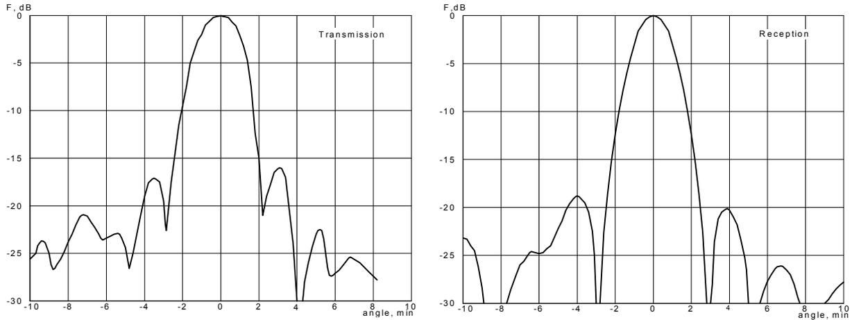
**Fig. 5.** Radiation patterns in broadside beam position
