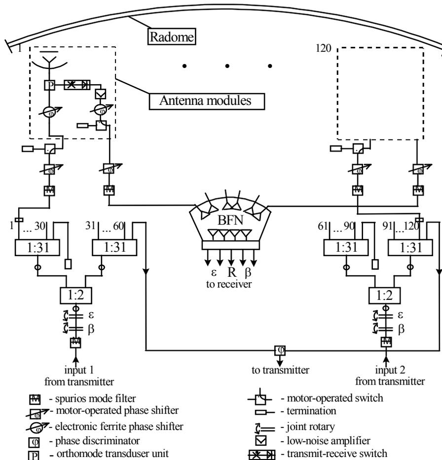
**Fig. 2.** The simplified block-diagram of antenna.
