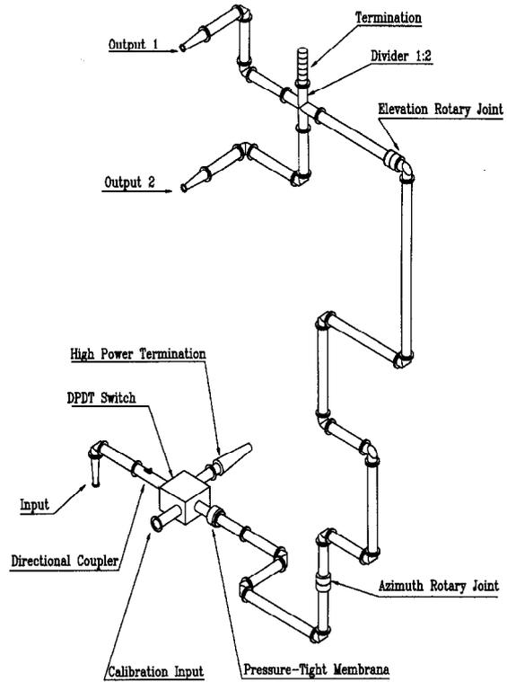
Fig. 6. Scheme of waveguide line from transmitter to two subarrays
