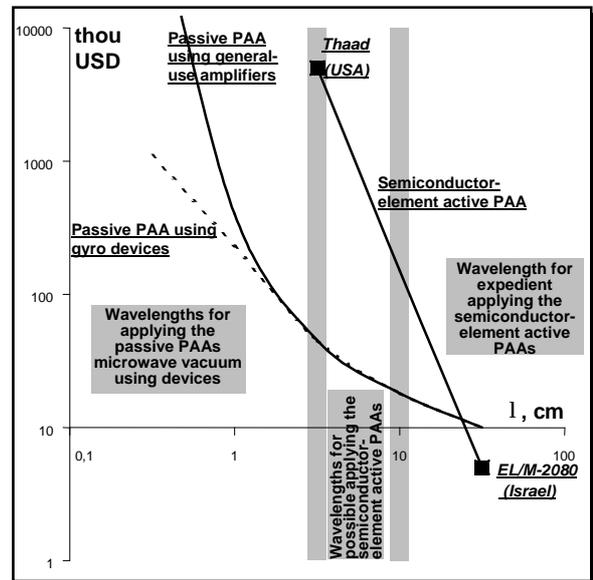
Fig.4. Cost of one sq.m of PAA aperture radiating 2 kW average power as a function of wavelength
