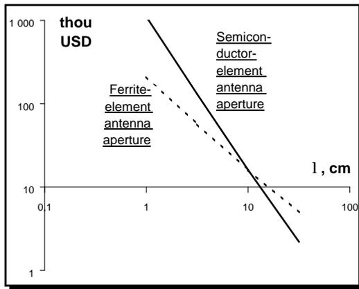
Fig.2. Cost of one sq.m of passive PAA aperture as a function of wavelength
