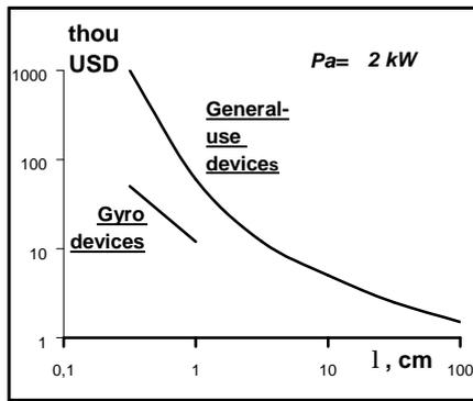
Fig.3 Cost of power amplification by means of different type microwave vacuum devices
