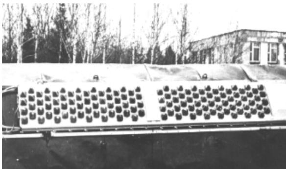
Fig. 9. L-band airborne APAA for communication system through the satellite “Molniya”
